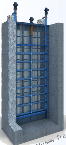
Shell Type Roller Gate
